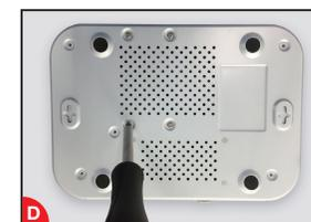
Holding the hard drive and the NVR, gently turn it over and line up the holes on the hard drive with the holes on the NVR. Using a Phillips screwdriver, screw the provided screws into the holes. Assemble the cover.
