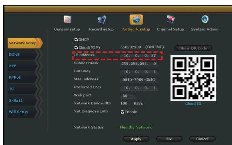
**Step2:** Enter the NVR's IP address in your IE browser in format http://your ip address, for example: http://10.0.0.37 (If the default WEB port 80 has been changed e.g. to 100, you'll need to add new port number when input IP address in the browser, for example: http://10.0.0.37:100)
