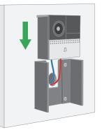
Insert the battery compartment into the doorbell.
